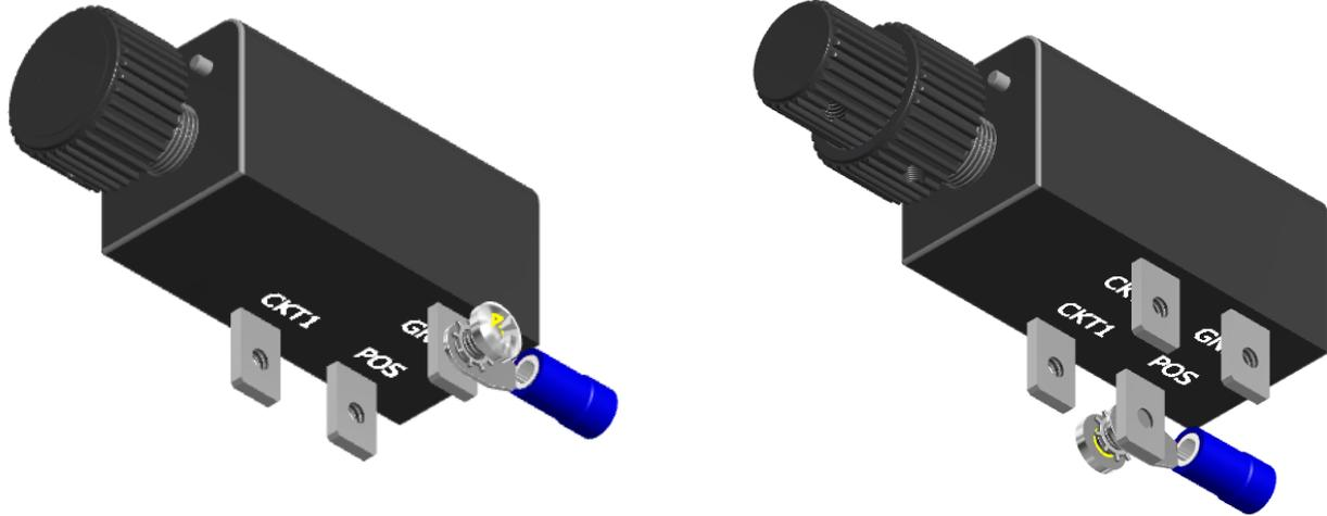
Shown are the two+ new dimmers from MaxPulse MaxDim. A Single output on the left, and a dual output on the right. The plastic is .9" square by 1.9" long. The terminals exit on one side and add .3" in one direction. The bushing is 6mm or 11mm long. Knobs are furnished with the units. What is different is the ability to have the units configured to your requirements.
